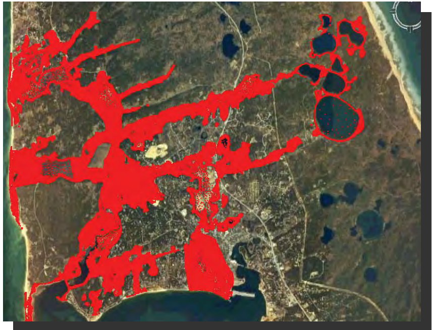
Figure ES-2. Elevation data from photogrammetric survey collected in 2007. Each red dot represents a data point.
