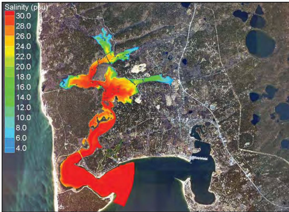
Alternative C: New Tide Control Structure at Chequessett Neck – Dike at Mill Creek that Excludes Tidal Flow
